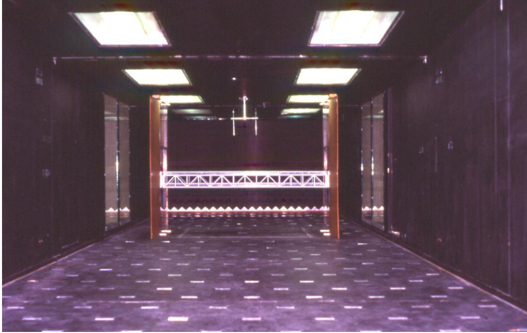
Figure Q.6 – Test on a bridge deck sectional model.
