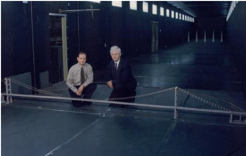
Figure Q.7 – Test on an aeroelastic replica model of a suspension bridge.
