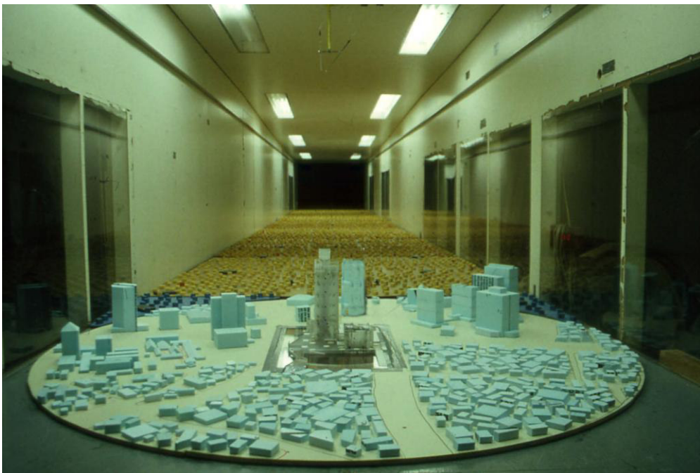
Figure Q.4 – Pressure test.
